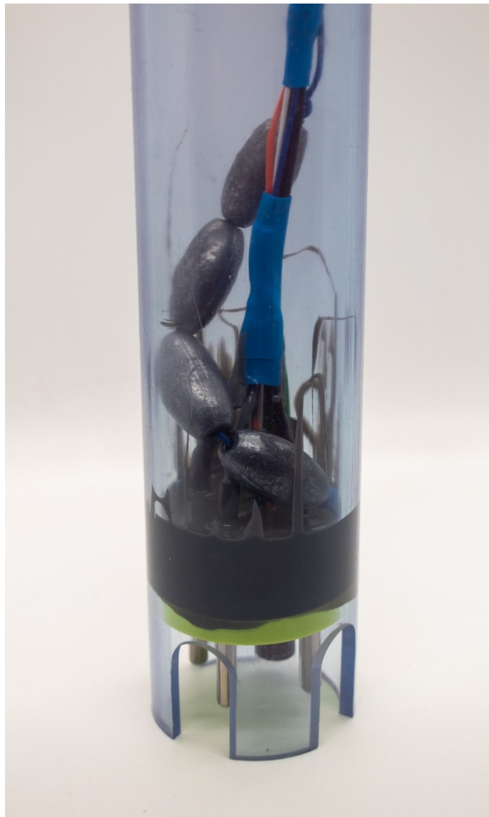
Figure 30. Clear OpenCTD with fishing weights inside.
