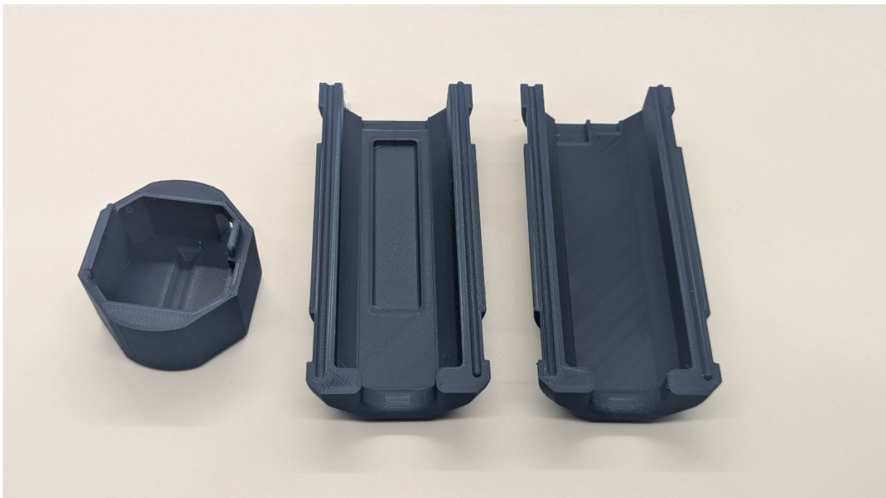
Figure 15: 3D-Printed chassis for OpenCTD.
