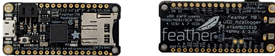
Figure 2. Adalogger M0 without headers. Left: topside of the board. Right: bottom of the board.
