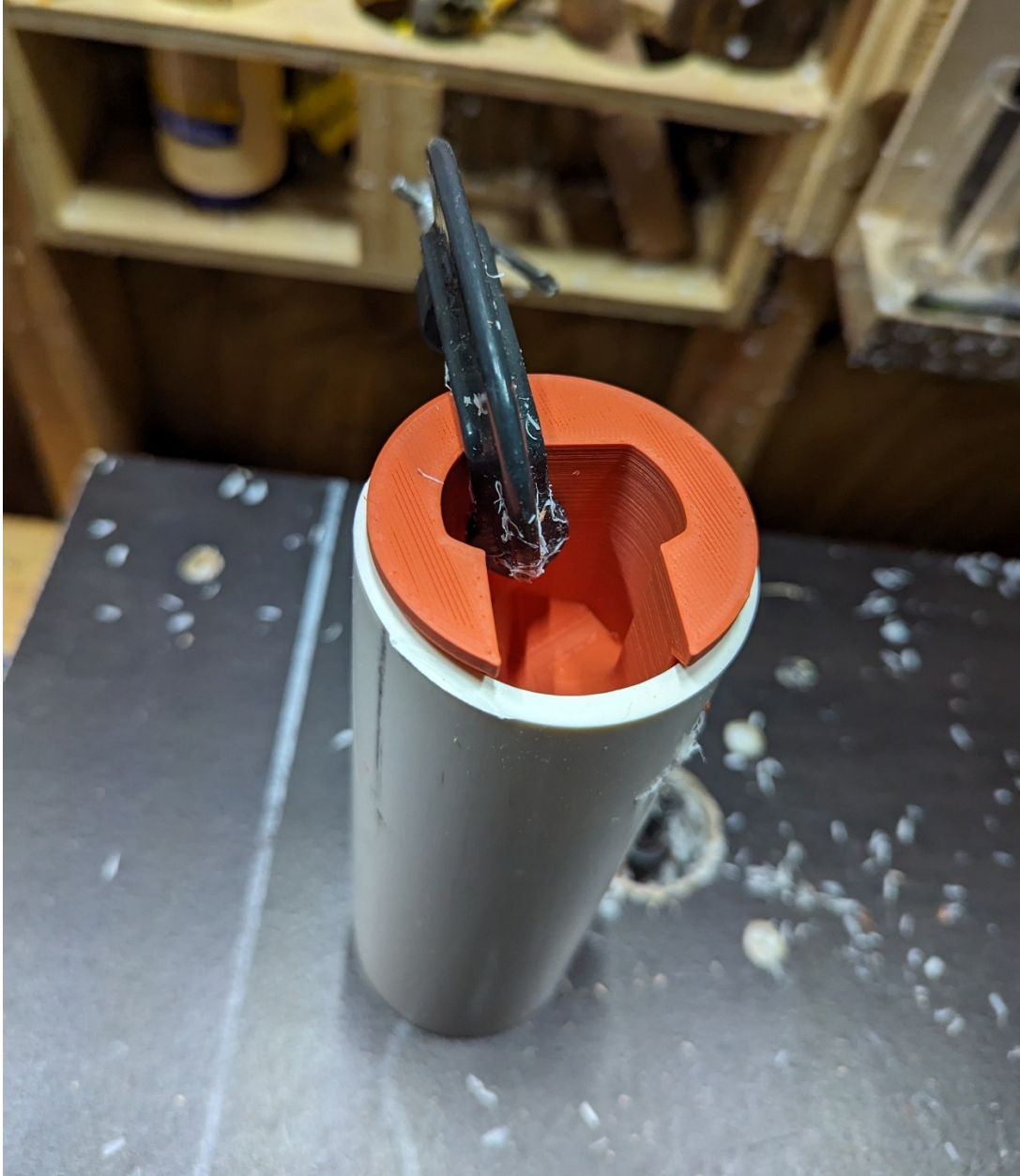
Figure 17. Router jig inserted into PVC pipe and secured with c-clamp.
