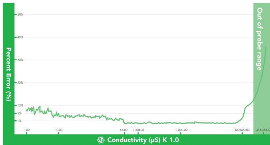
Figure 25. Accuracy of Atlas Scientific K 1.0 Conductivity Probe and EZO circuit. Data provided by Atlas Scientific.
