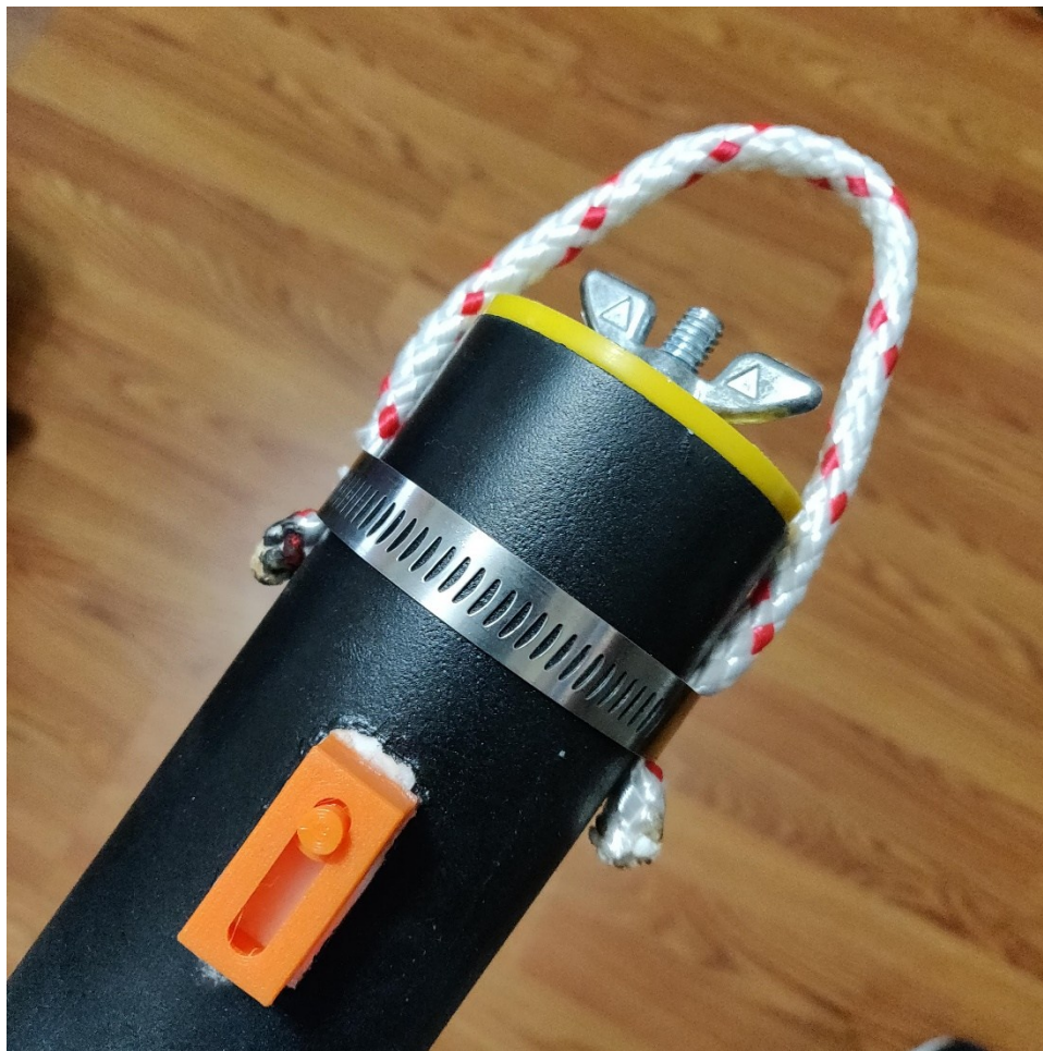
Figure 28. Finished OpenCTD with optional casting loop.
