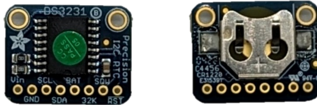
Figure 6. Real-Time Clock module without headers. Left: chip side of the board. Right: battery side of the board.
