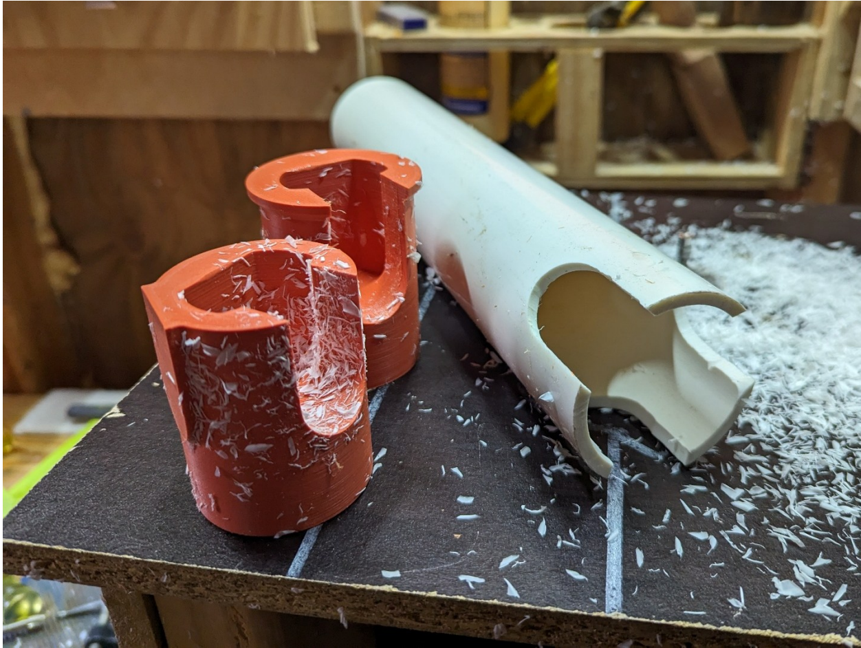
Figure 20. Completed PVC housing made on a router table.
