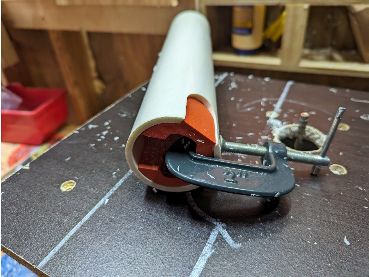
Figure 19. The second router jig inserted into the PVC pipe and secured with a c-clamp.
