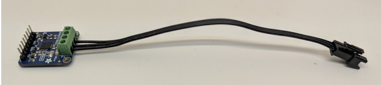
Figure 10. Completed MAX31865 amplifier with 3-pin connector cable installed.
