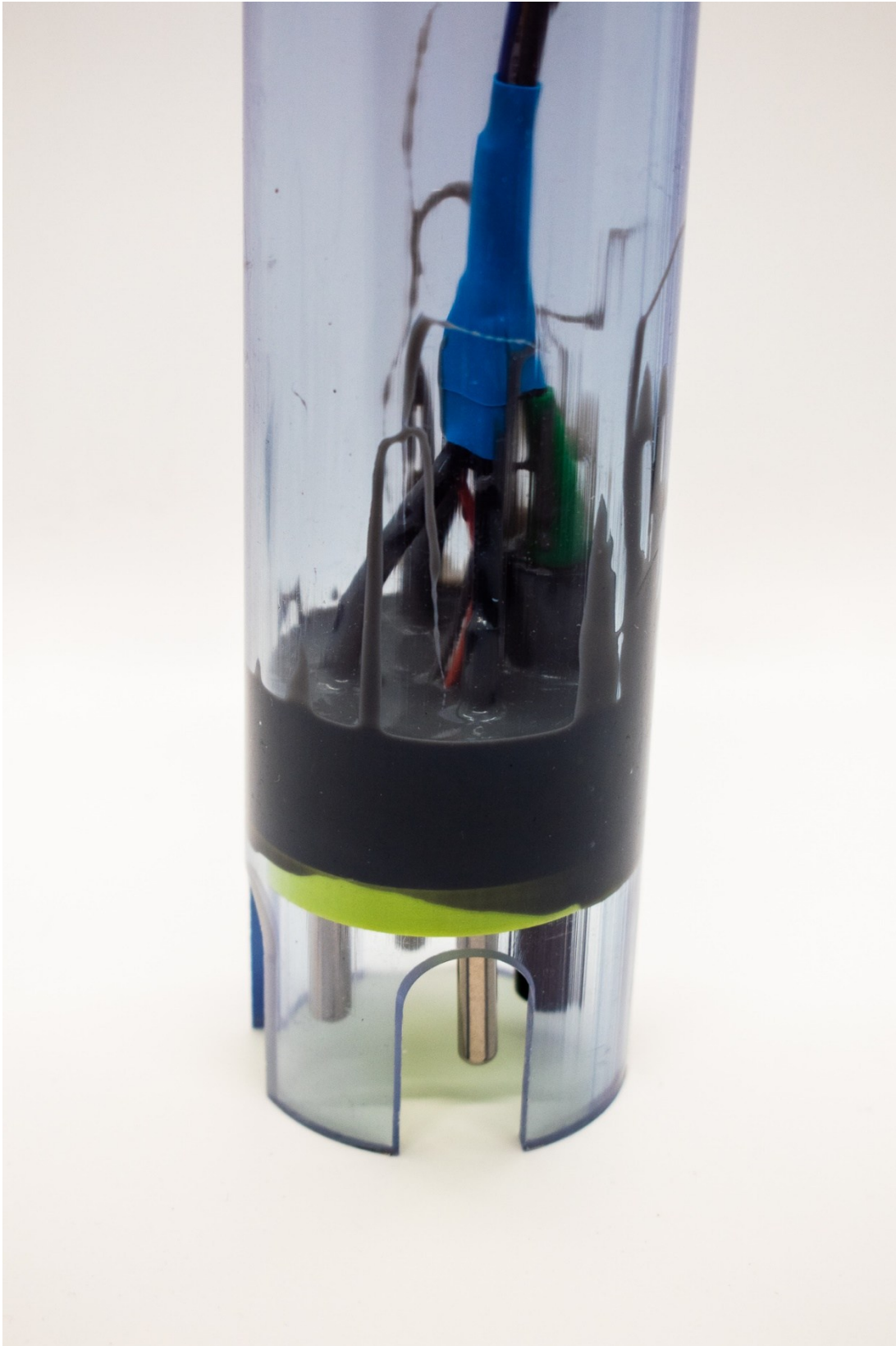
Figure 23. A clear OpenCTD showing the thick epoxy potting layer.
